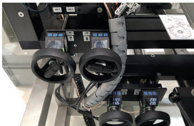
Figure 5: Size changeover using SIKO position indicators on a Track & Trace system in pharmaceutical manufacturing
