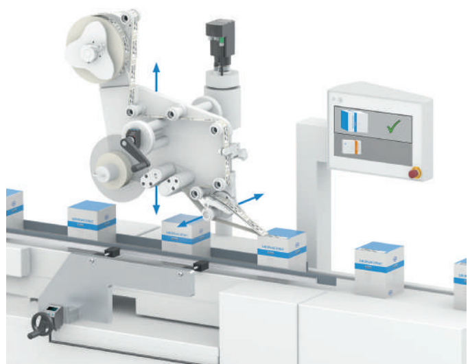
Figure 1: Size changeover using a labeling machine in pharmaceutical manufacturing
